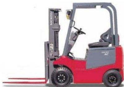
Gambar 2. Forklift elektrik Nichiyu FB20-75C
