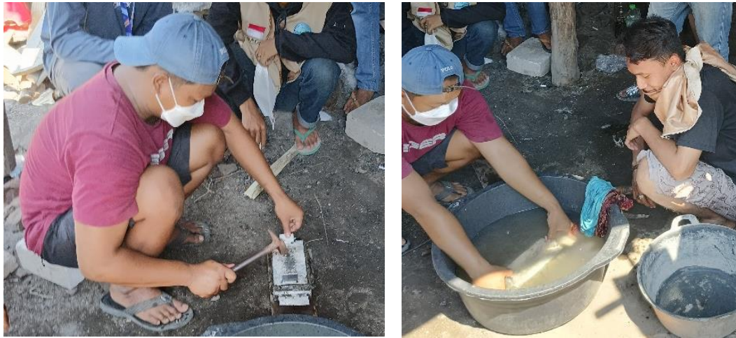
Gambar 4. Proses Pencetakan Paving Block
